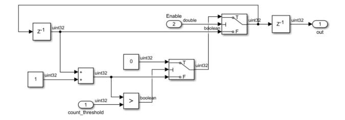
The Enable signal specifies whether the counter should count upwards from the previous value. When the Enable signal is logic high, the counter counts up from zero to the count\_threshold value. When the value of out becomes equal to the count\_threshold value, the counter wraps back to zero and starts counting again. When the Enable signal becomes logic low, the counter holds the previous value.
