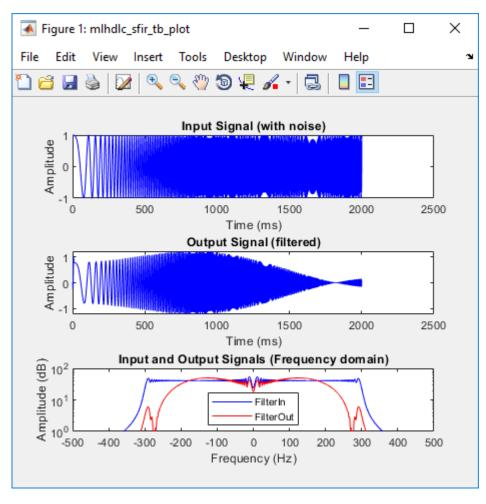
The test bench runs and plots the input signal and the filtered output.
